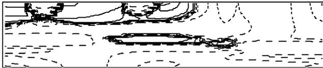
**Figure 2.** Values of  $d\mathcal{J}/d \ln k$  at each point in the domain as computed with the adjoint algorithm. The absolute values are not important since this is an artificial problem.
