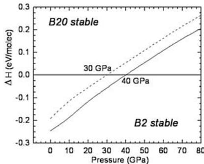
**Figure 1.** Enthalpy difference between the B20 and B2 structures in LDA (dashed line) and GGA (solid line).
