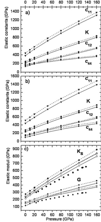
**Figure 2.** Pressure dependence of the elastic constants of FeSi in the B20 (a) and the B2 (b) structures, within LDA (dashed line) and GGA (solid line).  $K_s$  is the single crystal bulk modulus. c) Comparison between the isotropic polycrystalline aggregate elastic moduli for B20 (open symbols) and B2 (solid symbols) structures in LDA and GGA and PREM (symbols only).
