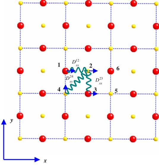
FIG. 1. (Color online) Schematic representation of the three largest force constants of periclase in  $xy$  plane: the Mg-O nearest-neighbor longitudinal interaction  $D_{xx}^{12}(V)$ , the Mg-O nearest-neighbor transverse interaction  $D_{xy}^{24}(V)$ , and the Mg-Mg nearest-neighbor interaction  $D_{xx}^{23}(V)$ . Oxygen and magnesium are represented by large (red) and small (yellow) spheres, respectively.
