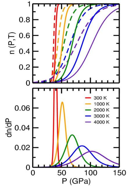
FIG. 6. (Color online) (a) LS fraction,  $n(P, T)$ , of Fp with  $x = 0.1875$  as a function of pressure along several isotherms. The figure presents the results with (full lines) and without (dashed lines) including the vibrational contribution to free energies. (b) Derivatives  $\partial n / \partial P$  at the same temperatures as (a).
