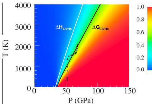
FIG. 5. (Color online) “Phase diagram” of Fp with  $x=0.1875$ . The black and white lines correspond to the middle point of the crossover, where  $n(P, T)=0.5$ , computed with and without including the vibrational contribution to the free energy, respectively. The plus symbols are experimental data corresponding to  $n=0.5$  (Ref. 9).
