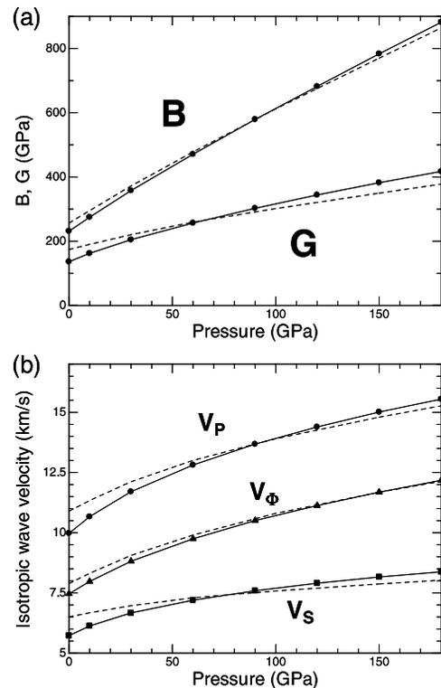
**Figure 2.** Pressure dependence of the aggregate properties of post-perovskite (solid lines) compared with those of perovskite (dashed lines). (a) Bulk and shear moduli. (b) Compressional, shear, and bulk isotropic wave velocities.
