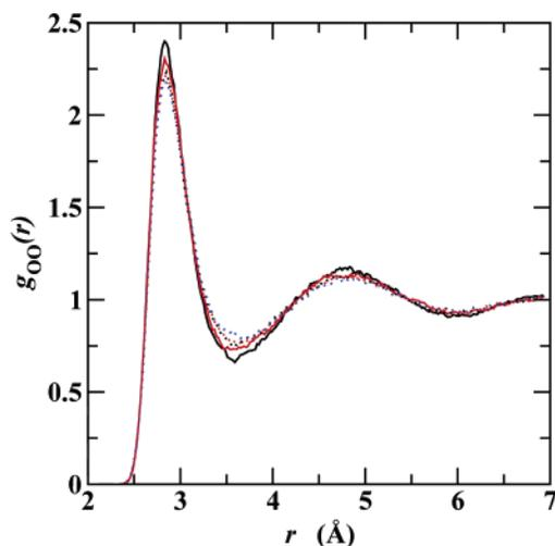
**Figure 2.** The oxygen–oxygen radial distribution functions obtained from molecular dynamics simulation of water using the BLYP exchange/correlation energy functional at  $T = 423$  K and  $\rho = 0.71$  g  $\text{cm}^{-3}$ . The lines correspond to (refer to text for descriptions) the following: BO-1 (black, solid), BO-2 (red, solid), CP-100 (black, dot), CP-200 (red, dot), and CP-300 (blue, dot).
