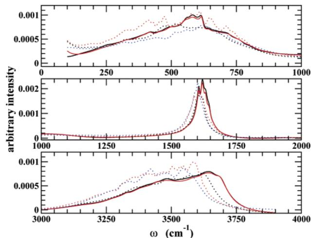
**Figure 9.** Power spectra computed from the regularized resolvent transform of the total velocity autocorrelation function.<sup>36,37</sup> The spectrum is divided into three regions (from top to bottom: librations, bending motion, and stretching modes) for clarity. The line styles and colors are the same as Figure 2.
