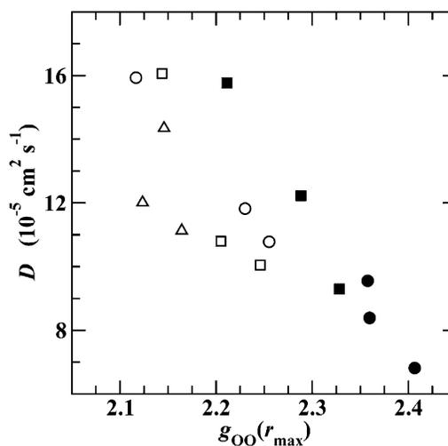
**Figure 5.** The diffusion coefficient as a function of the peak height of the first maximum in the oxygen–oxygen radial distribution function. Data points were obtained by dividing the simulations into three parts of equal length and computing the values for these segments. The runs are as follows: BO-1 (solid circle), BO-2 (solid square), CP-100 (open circle), CP-200 (open square), and CP-300 (open triangle up).
