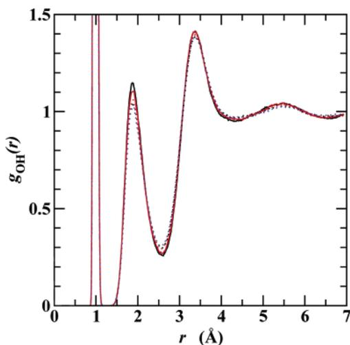
**Figure 3.** The oxygen–hydrogen radial distribution functions obtained from molecular dynamics simulation of water using the BLYP exchange/correlation energy functional at  $T = 423$  K and  $\rho = 0.71$  g cm $^{-3}$ . The line styles and colors are the same as Figure 2.
