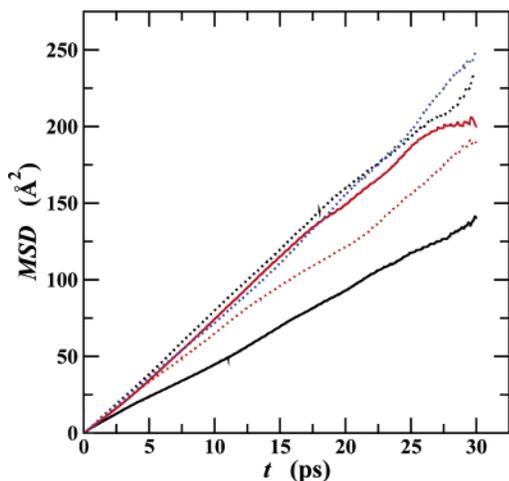
**Figure 4.** The mean squared displacements obtained from molecular dynamics simulation of water using the BLYP exchange/correlation energy functional at  $T = 423$  K and  $\rho = 0.71$  g cm $^{-3}$ . The line styles and colors are the same as Figure 2.
