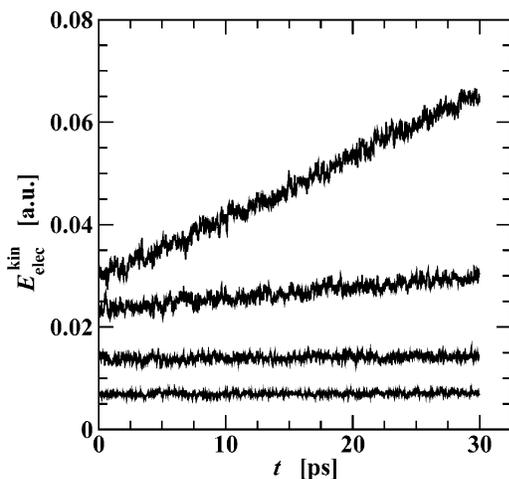
**Figure 1.** The instantaneous fictitious electronic kinetic energy as a function of time for all four Car–Parrinello molecular dynamics simulations. From top to bottom: CP-400, CP-300, CP-200, and CP-100.
